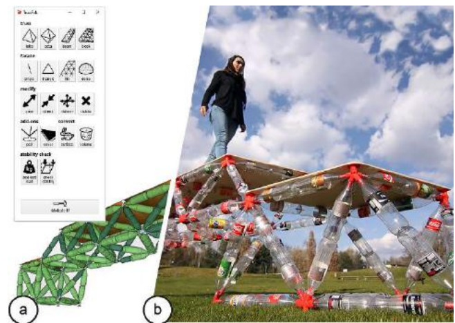
Figure 1: TrussFab is a system that allows users to fabricate large structures sturdy enough to carry human weight. TrussFab considers bottles as beams that form structurally sound node-link structures also known as trusses , allowing it to handle the forces resulting from scale and load.
