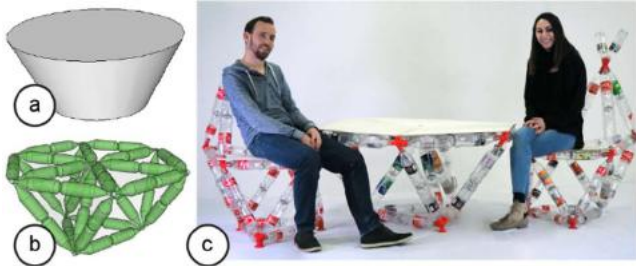
Figure 2: (a) TrussFab’s converter automatically turns this 3D model of a coffee table, into (b) a sturdy tetrahedral honeycomb structure, (c) which fabricated serves as a functional table.
