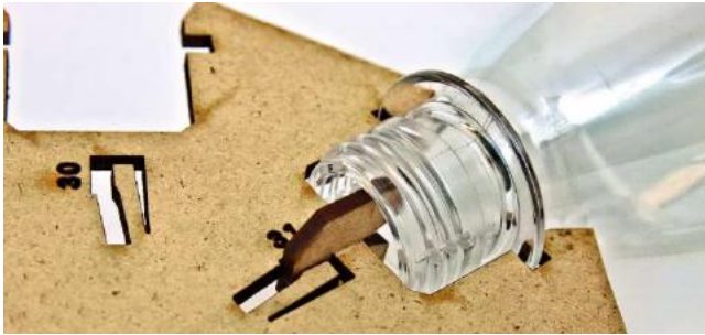
Figure 17: Laser-cut snap connectors are secured using a self-locking wedge.
