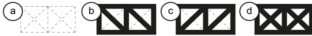
Figure 3: (a) The basic grid structure allows reinforcing rigid member cells (b-c) with one diagonal or (d) two diagonals.
