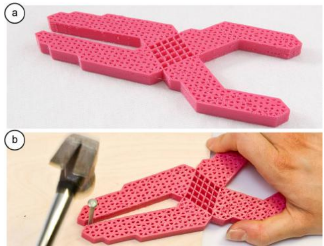
Figure 10: (a) This pair of pliers is based on a single metamaterial four-bar. (b) When the user applies a force to the handles, the hinge array in the center transmits this force to the brackets, and the pliers close.
