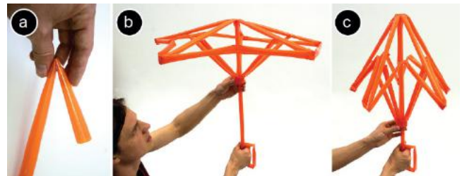
Figure 5: (a) Protopiper allows creating simple mechanisms, such as hinges that allow opening-closing an umbrella (b, c).
