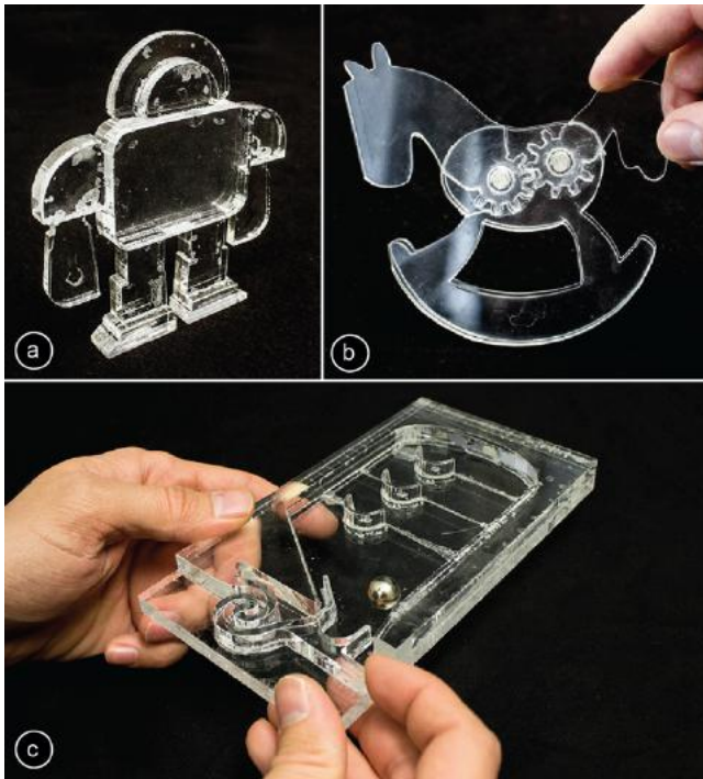
Figure 12: Different classes of objects: (a, c) pyramid shapes do not require healing. (b) Other shapes require healing. The little robot and the mechanical horse toy take 2.5 min to fabricate, while the pinball table takes 14 min due to its thicker layers.
